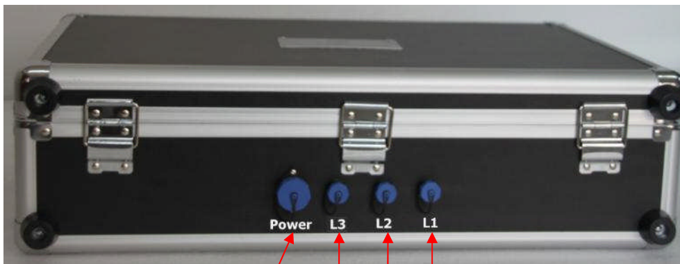
Main Power & L3 L2 L1 Current Clamps Socket Power
